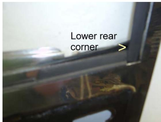
The metal channel does **not** have the inner lips like at the bottom rear corner. Hence, it is not necessary to change the width at the top. Finish both ends and install this piece. It will fit very tight in the metal channel. (note: I did not use weather strip adhesive).
